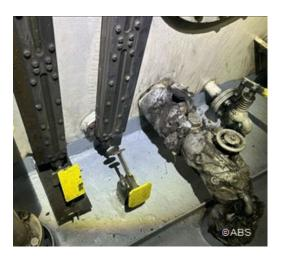
Quick closing valves for lubricating oil system and marine gas oil system blocked permanently in open position.
