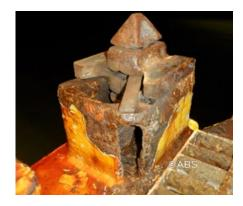
Twist lock foundation at container housing cracked
