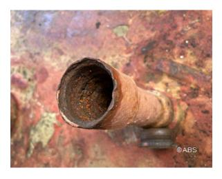
Sounding pipe closing cap thread damaged
