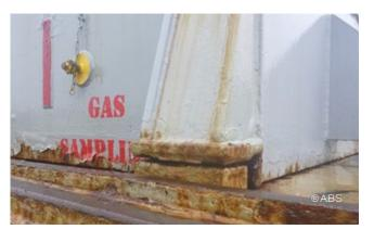
Hatch cover support pads with excessive wear, over compressed weathertight gasket and panels resting on coaming
