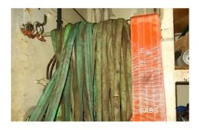
Safe operating load markings missing for slings
